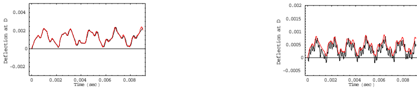
Figure.6. Deflection at node D of 4-step CC beam when subjected to step load of 1000N at node A when thickness of beam ( h ) changes from 3.97mm to 5.56mm. (Left picture for when thickness is 3.97mm and right picture for when thickness is 5.56mm) It seems that the step load affects fourth mode eigenfrequency in Timoshenko Model——— . Euler Bernoulli Model——— .
