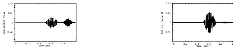
Figure.9. Deflection at nodes A and B of 3-step CC Timoshenko beam with thickness of 5.56mm when it is subjected to a sinusoidal load of 100N at 0.05m from left side with duration of 0.2 sec.
