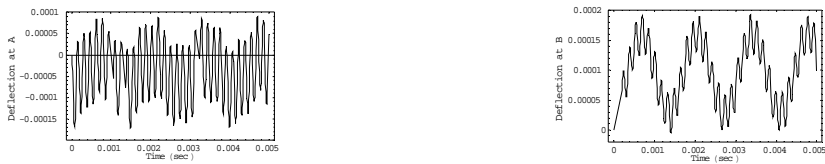
Figure.7. Deflection at nodes A and B of 3-step CC Timoshenko beam with thickness of 5.56mm when it is subjected to a step load of 100N at 0.05m from left side.
