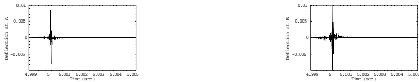
Figure.8. Deflection at nodes A and B of 3-step CC Timoshenko beam with thickness of 5.56mm when it is subjected to a ramp load of 100N at 0.05m from left side with duration of 0.003 sec.
