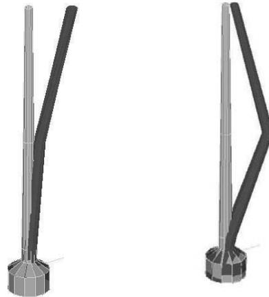
Figure 11 mode shape for first (left) and second (right) natural frequency.
