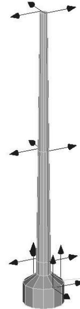
Figure 9 Location and orientation of sensors (green arrows)
